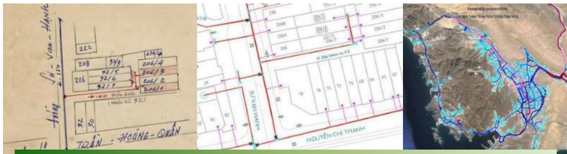
Example of network structure digitized from paper to GIS and then to hydraulic model
