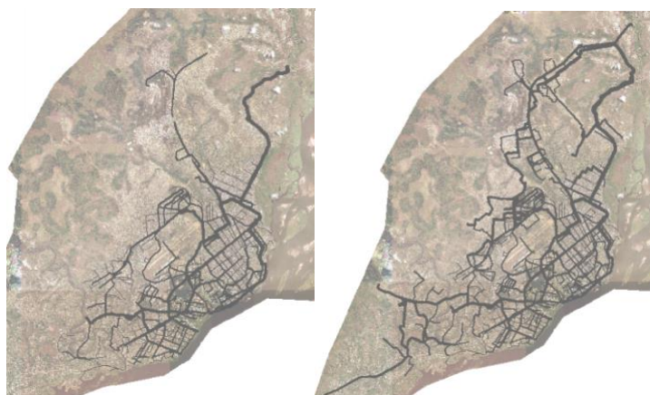
Example of hydraulic model refining over time to include smaller distribution mains
